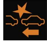
Forward Collision Warning/Collision Mitigation Braking System Indicator
