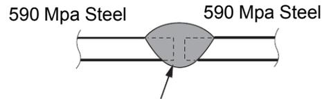
Wire tensile strength must be  $\geq 590$  MPa (86 ksi)
